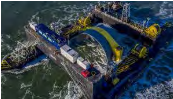
Figure 1. Tidal turbine sits in a barge in preparation for deployment, November 7, 2016, in Minas Passage, Nova Scotia.
